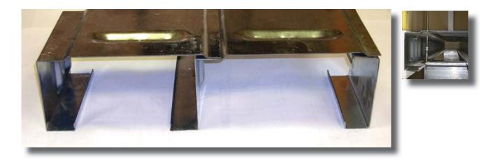
Angle Cuts. You can design your deck with curves or angles, similar to wood structures. Actually, the 39-inch cantilever with our system is an advantage when designing curves or angles. The steel structure may be cut either before or after assembly using a standard skilsaw with a metal-cutting blade (such as Diablo brand).
