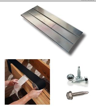
**INSTALLATION.** PAVERDECK<sup>tm</sup> planks may be installed over standard wood or steel joist supports designed in compliance with applicable building codes. When installing PAVERDECK<sup>tm</sup> planks over treated wood supports, an isolation gasket / moisture barrier is required between the steel and the treated wood (eg. Deckwise Tape, peel/ stick moisture shield etc.).
